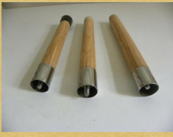
Once you have established this you can put it back on the lathe and reduce the stick to the required height before turning the diameter down to take the Rubber Foot. Photo below is the finished article.
