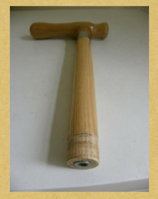
Making certain the stick screws together properly before gluing once satisfied glue both the studding and the Ferrell on the top of each remaining piece.
