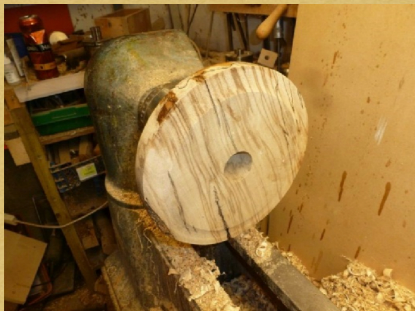
Image 3: Bowl mounted on spigot.
