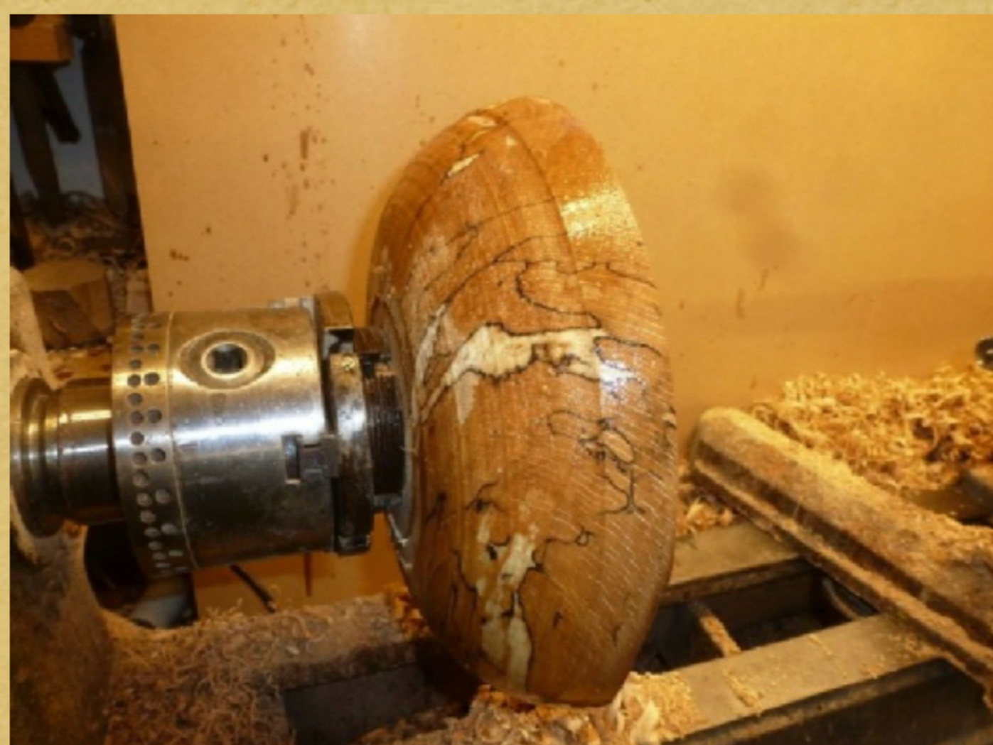
Image 5: Coating of sanding sealer.
