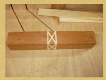
completed The blank after all four cuts and joints completed and faces cleaned up with a sharp plane / sandpaper
