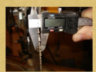
Measuring the saw blade and veneer. Remember that you need to measure the width between the tips of the saw teeth.
