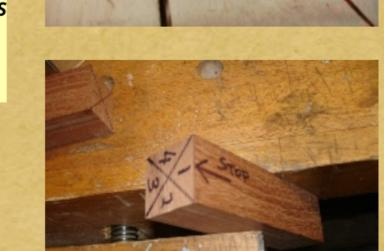
Now draw diagonals across each end to find the centre of your blank and mark one end to be the "stop end." Now, looking at the stop end, number the faces of the 1 to 4 working in a clockwise direction.
